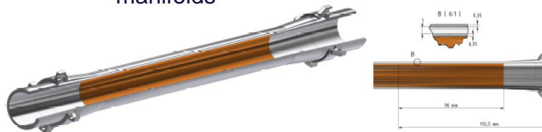
Fig. 48: Central chamber in AlBeMet162 including cooling inlets and outlets (left); cross- and zoom of the structure of the cooling channel for the paraffin flow.
