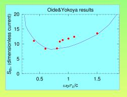
Threshold current as a function of  $\omega_0$ , Q=1.
