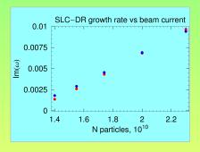
Wakefield for the SLCDR and comparison of the new code (blue dots) with the published results (red dots). The growth rate  ${\rm Im}\,\omega$  is in units  $\omega_{s0}$ . The radiation damping in the ring is  $\gamma\approx 0.001\omega_s$ .
