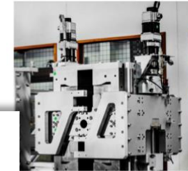
Photograph of a ZEPTO tuneable permanent magnet dipole at Diamond Light Source
