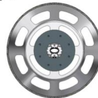
Centered position for pipe insertion
