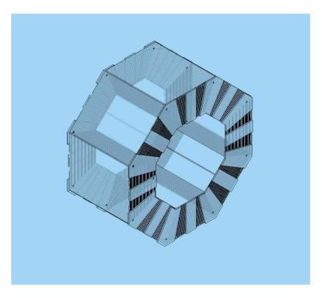
The only input (so far) is enough steel to nominally return the flux, and 10 cm laminations w 5 cm gaps all the way through. The gaps make the radiation physicists looking at self-shielding nervous! We should collapse the un-needed gaps in the next iteration - how about 3 stations of 2 gaps for muons??
