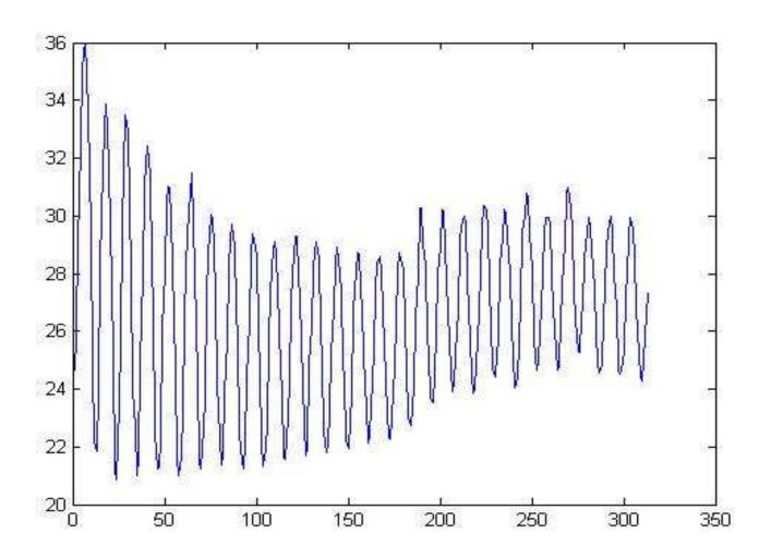
This is dispersion uncorrected emittance. Hence, real mode emittance is less than the minima.
