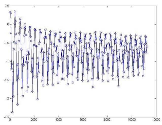
Dispersion calculation in LIAR is incorrect (sign problem in SBEND) Fix is being worked out
