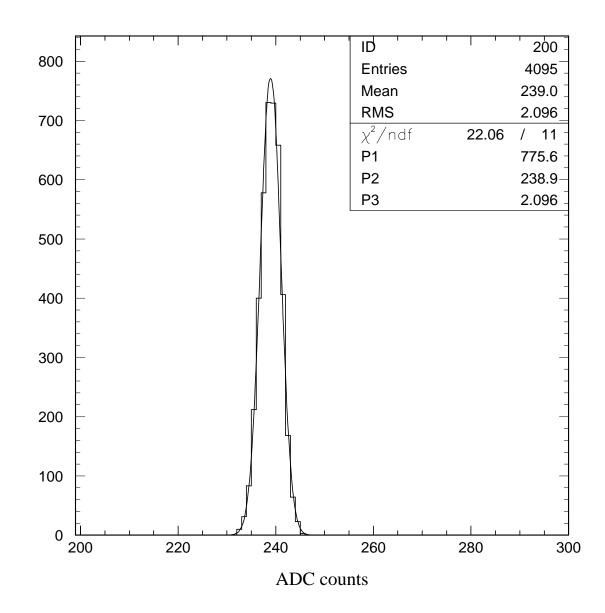
Typical noise in the ADC corresponds to less than 1 fC.
