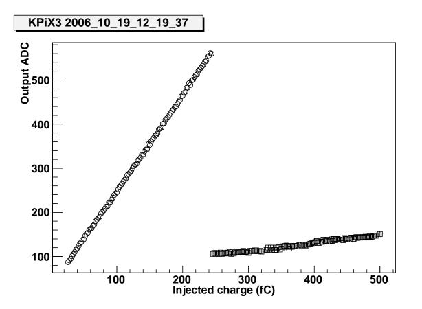
Range switching level adjusted to occur at 200 fC rather than 400 fC for illustration.
