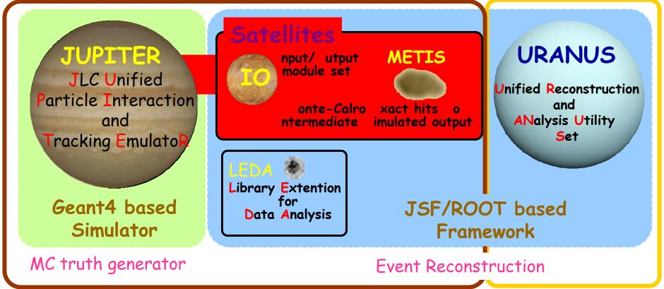
JSF: the analysis flow controller based on ROOT The release includes event generators, Quick Simulator, and simple event display
