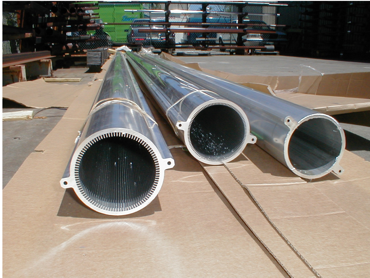
Extruded aluminum beam pipe with "fins" and coating.
