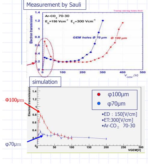
The figure shows transmission as a function of VGEM for Ar:CO2=70:30, where Ed is set to 150V/cm and Et is set to 300V/cm.
