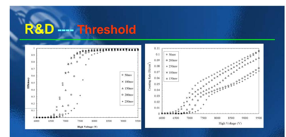
Efficiencies versus high voltage for different discrimination thresholds Singles counting rates versus high voltage for different discrimination thresholds
