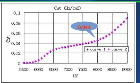
The Efficiency is about 97% The Dark current is about 1µA The Single counting rate is about 0.05Hz/cm<sup>2</sup>
