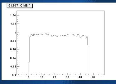
Module size: 3800mm\*1640mm Strip length: 3800mm Strip width: 33mm Average strip efficiency: 0.99 Spatial resolution: 14.2mm
