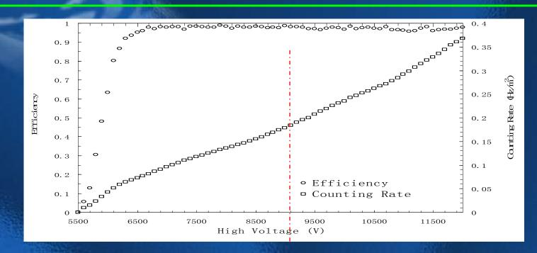
Efficiencies and singles counting rates versus the high voltage up to 12 kV. This plot shows the behavior of the prototype RPC under extreme high voltages. The gas mixture used was Ar/C2F4H2/C4H10 50:42:8.
