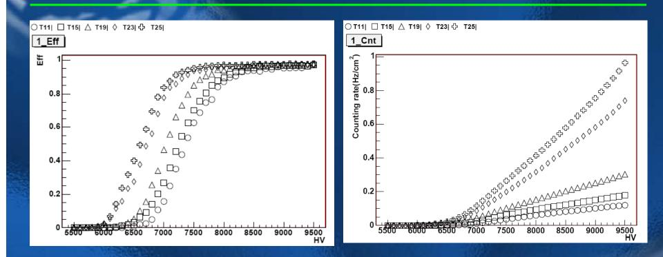
The efficiency and counting rate versus temperature. Efficiency curve will shift to left side at high temperatures, and the counting rate will increase exponent with temperature.
