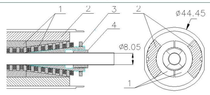
Details of design. 1–Iron yoke, 2–Copper collar, 3, 4–trimming Iron nuts. Inner diameter of Copper vacuum chamber is 8mm clear.
