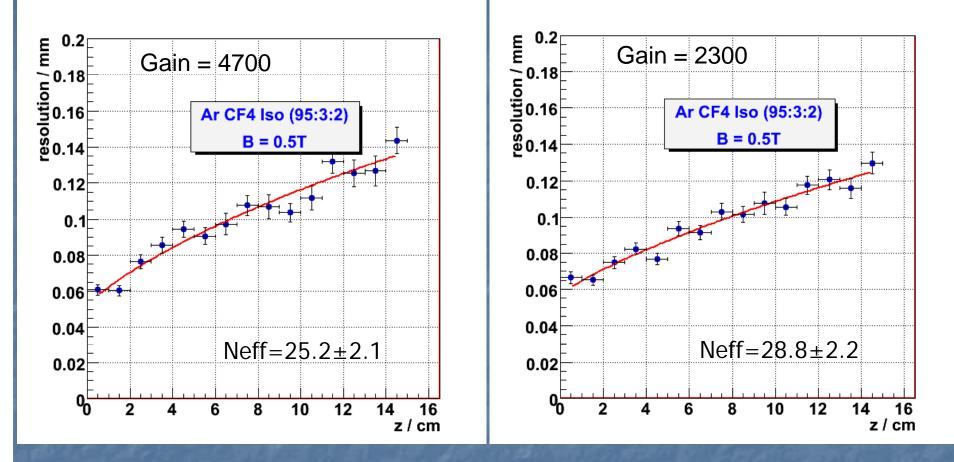
At 4 T with this gas, the point resol° is better than 80  $\mu$ m at z=2m Even higher B fields possible (A. Yamamoto): new concept?
