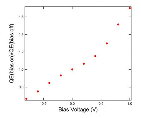
We clearly observe the bias effect on the qe after 1 hour of heat cleaning The cathode at 495C
