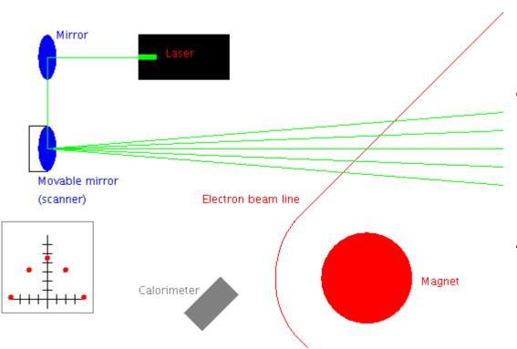
• The resolution of a laser-wire depends on the size of the laser beam
