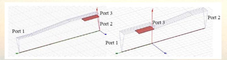
If an aperture restriction can be tolerated, the inner pipe may be inserted into the beam pipe and a taper added after the coaxial section.
