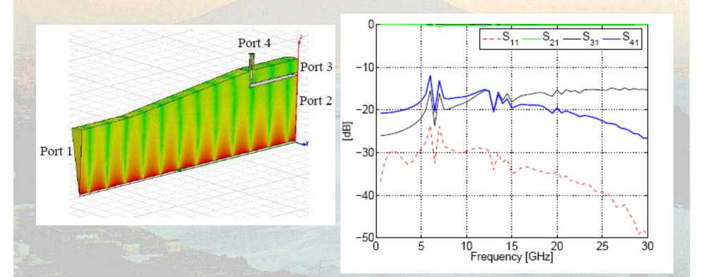
With the courtesy of Tom Kroyer ("A Structure for a Wide Band Wall Current Monitor", AB-Note-2006-040 RF)
