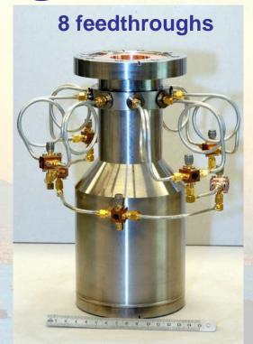
The existing design is based on a previous design for the CTF2 (63 MHz  $\leq$  bandwidth  $\leq$  10 GHz )
