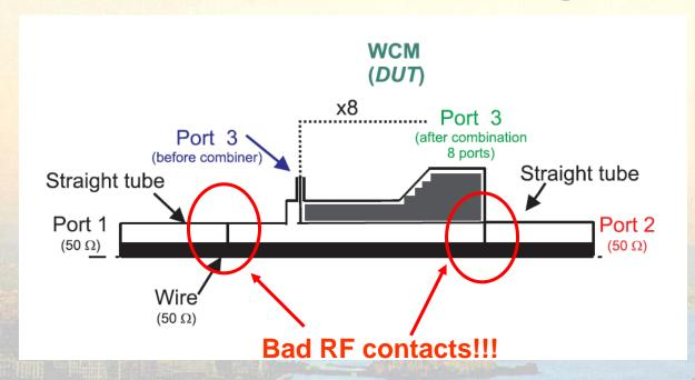
The experimental setup showed very bad RF contacts between WCM and the two external straight tubes. In order to improve the contacts some pasty stripes of conducting material has been used.... Unfortunately it cannot be used in vacuum....
