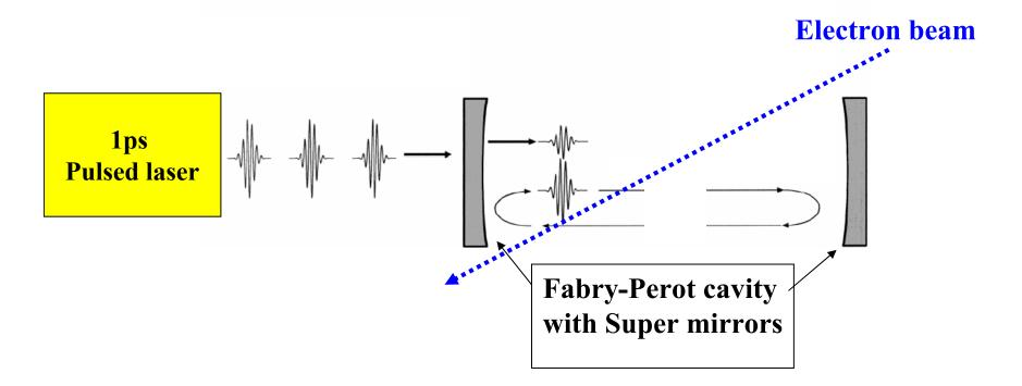
Pulse energy gain of the order of 10<sup>4</sup>-10<sup>5</sup> can be obtained inside the cavity for pulse width ~1ps..
