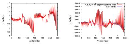
To minimise the emittance we should try to turn the left plot into a straight line by using the knobs k<sub>i</sub>
