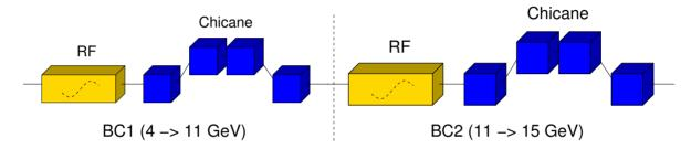
• Idea: off-phase beams gain different energy with respect to the nominal one  $\Rightarrow$  off-phase beams can be used as test-beams for the DFS in the Main Linac
