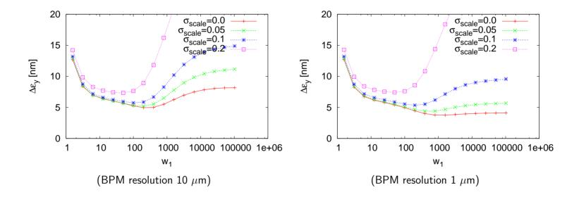
$\Rightarrow$  For large scale errors, the curvature does not allow to use large values of  $\omega_1$  and thus one does not take full advantage of the good BPM resolution
