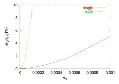
$\Rightarrow$  in green the emittance integrated over a few pulses and assuming that no feedback is used  $\Rightarrow$  the main contribution is due to trajectory jitter: a jitter of  $0.5\sigma$  leads to 12% growth
