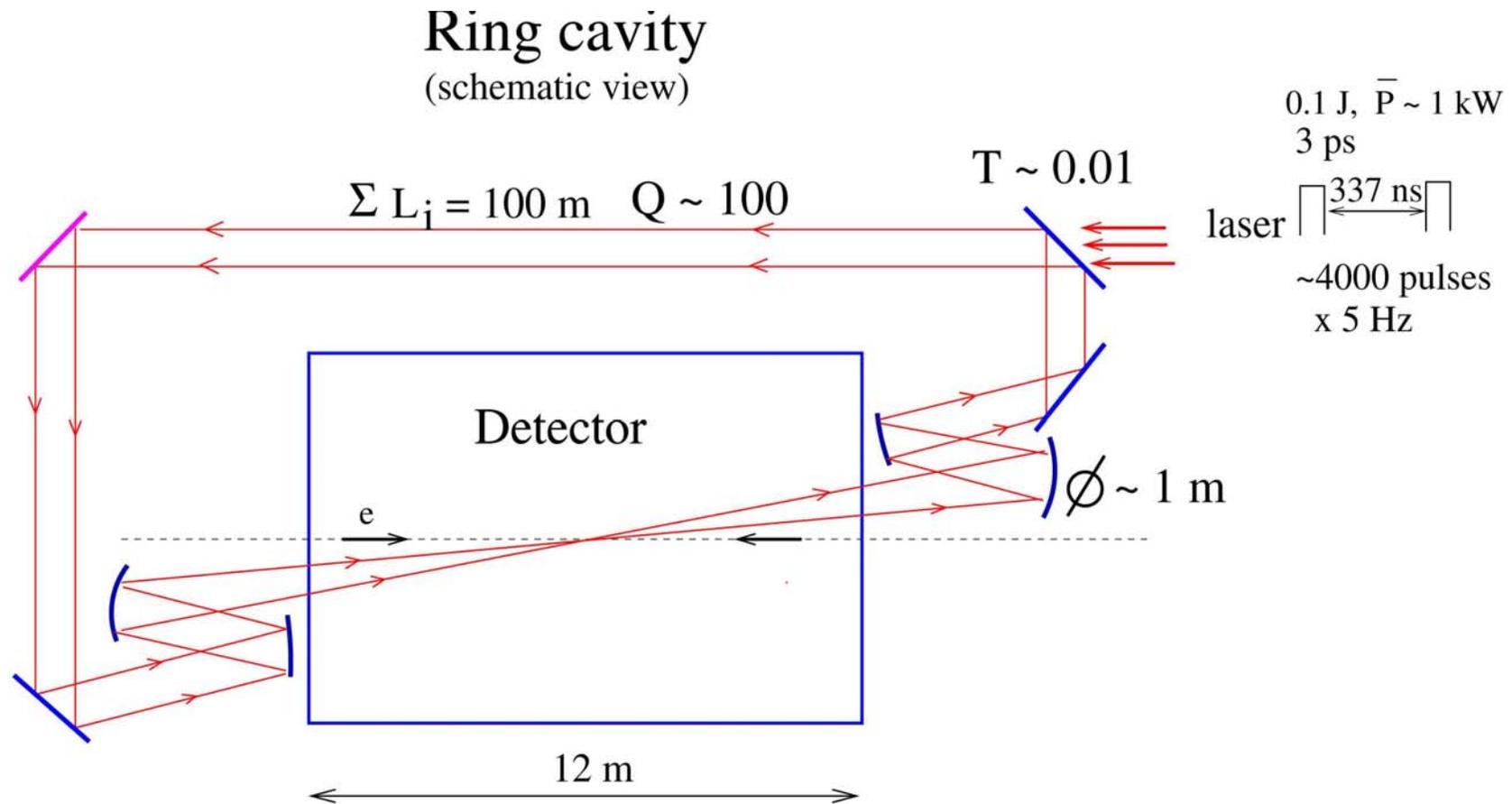
The cavity includes adaptive mirrors and diagnostics. Optimum angular divergence of the laser beam is  $\pm 30 \text{ mrad}$ ,  $A \approx 9 \text{ J}$  ( $k=1$ ),  $\sigma_t \approx 1.3 \text{ ps}$ ,  $\sigma_{x,L} \sim 7 \text{ } \mu\text{m}$
