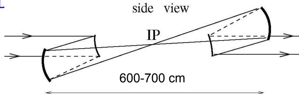
Then the diameter of focusing mirror is about 20 cm and that of the auxiliary mirror about 11 cm. The dead angle for tracking remains as before about  $\pm 95$  mrad, but smaller for calorimetry. The laser density is far below the damage threshold, the average power is the most serious problem.
