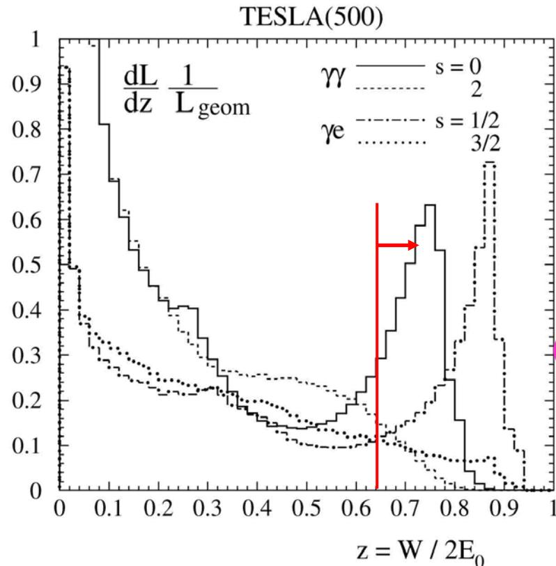
Usually a luminosity at the photon collider is defined as the luminosity in the high energy peak,  $z > 0.8z_m$ .
