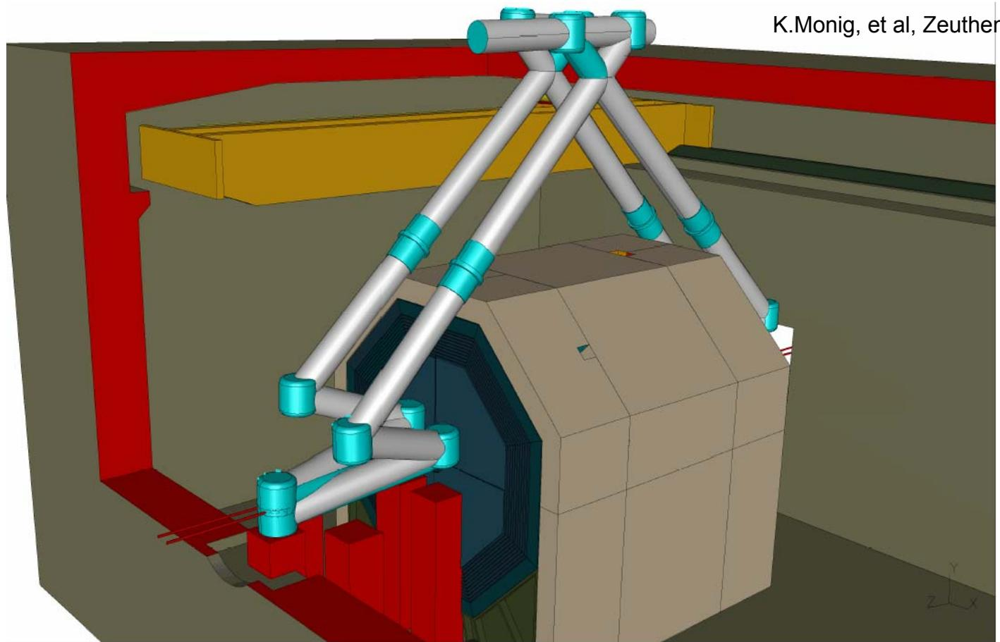
For easier manipulation with bridge crane and smaller vibrations it may be better to hide the laser tubes under the detector
