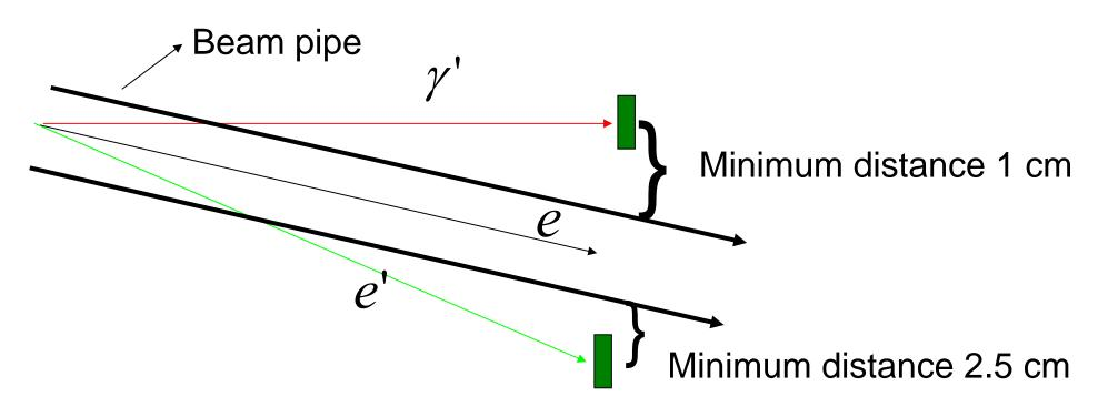
•We have some restrictions on the length L due to practical reasons, for example separation between beam and photons must be at least 20 mm if the beam pipe has a radius of 10 mm.
