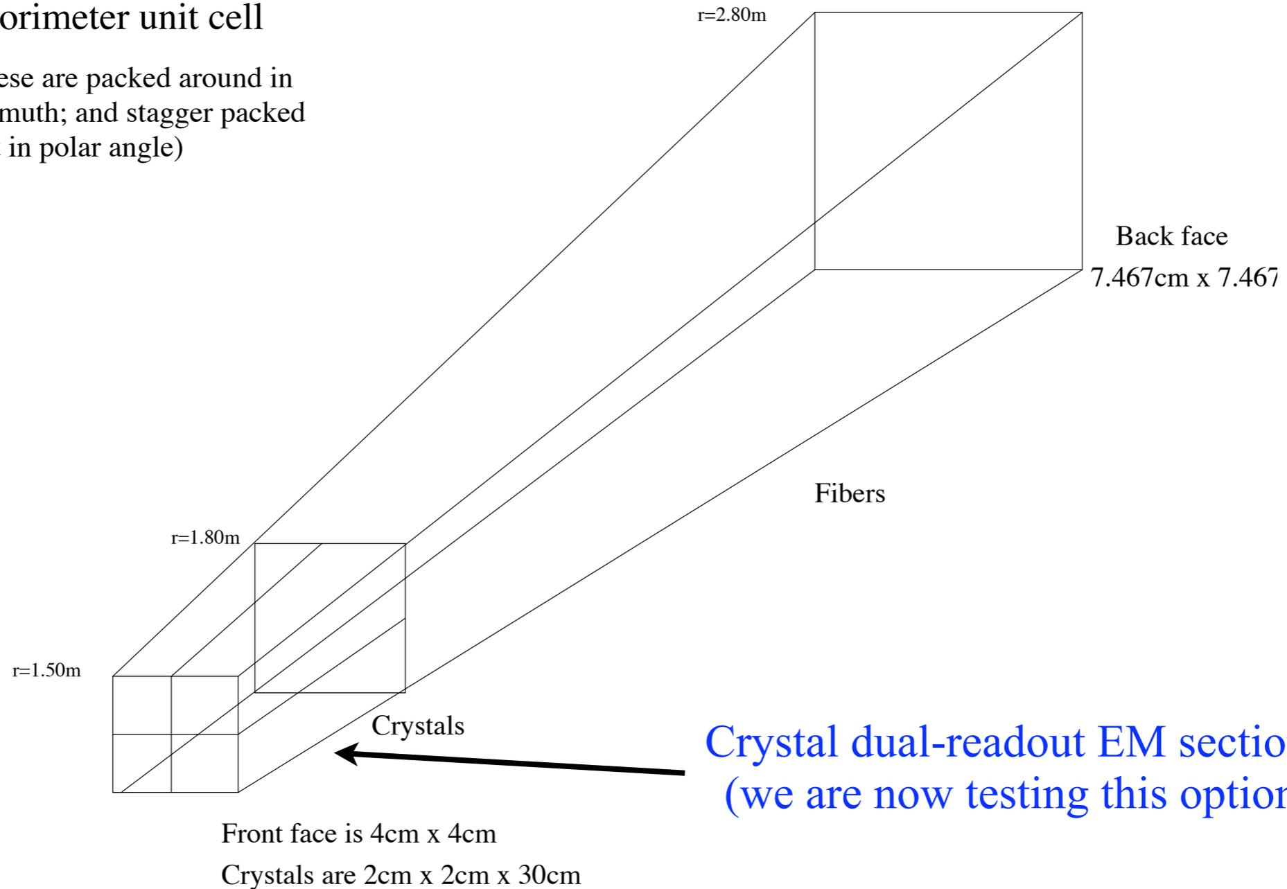
A “scalable” module; excellent electron & photon measurement; excellent hadron measurement.
