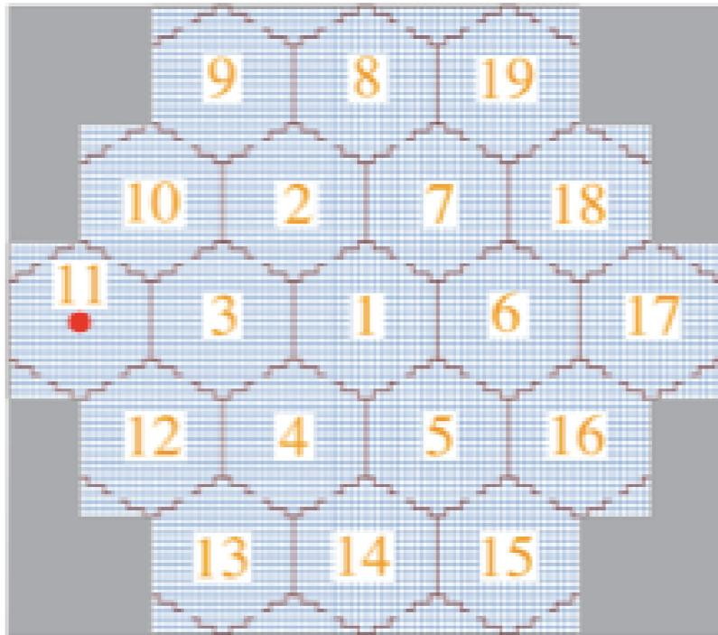
Send pion beam into center of channel 11, clock out scintillator/PMT signals in channels 3, 1, 6 and 17.
