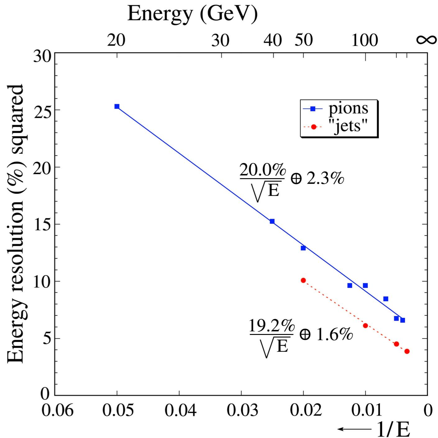
DREAM module calibrated with 40 GeV  $e^-$  into the centers of each tower responds linearly to  $\pi^-$  and “jets” from 20 to 300 GeV.
