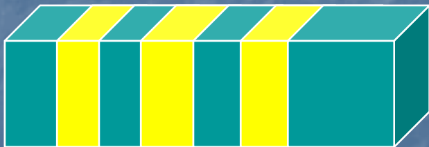
Longitudinally segmented calorimeter (plastic scintillator)
