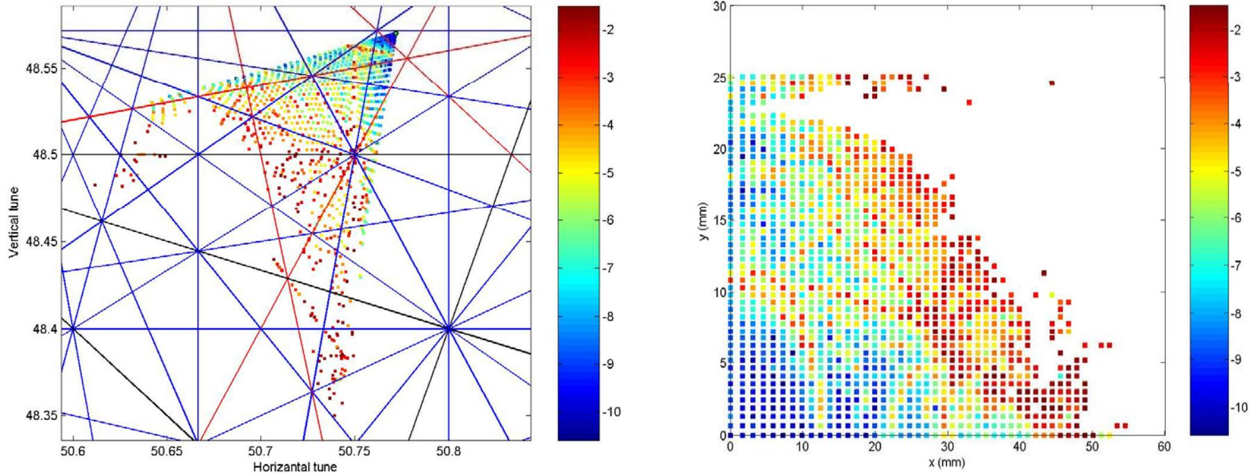
FMA analysis for on momentum particles: (Left) footprint; (Right) Dynamic aperture with FMA.
