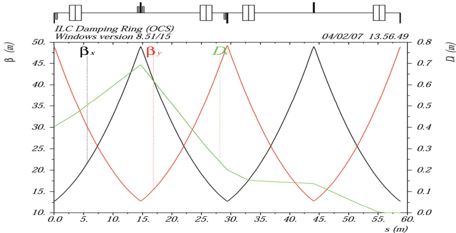
Add one arc cell after the last standard arc cell and **modify the bending angle** of these two cells according to the phase advance. The aim is to have undisturbed TWISS parameters in the dispersion suppressor.
