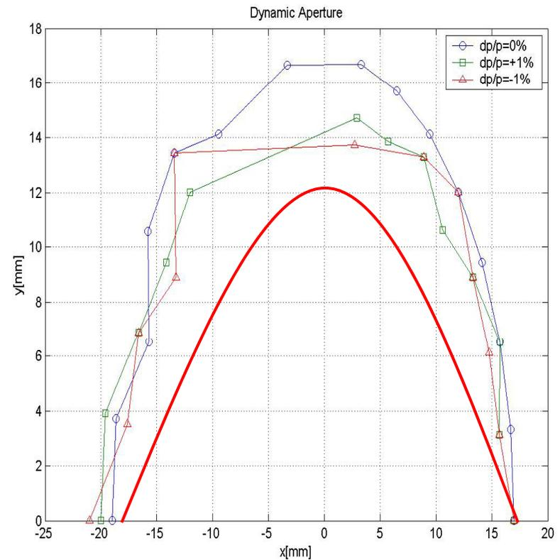
The chromaticity corrected to (0.15,0.15). The tune variation with momentum spread  $\pm 1\%$  ; the dynamic aperture with momentum spread up to  $\pm 1\%$  (with RF cavity, no errors).
