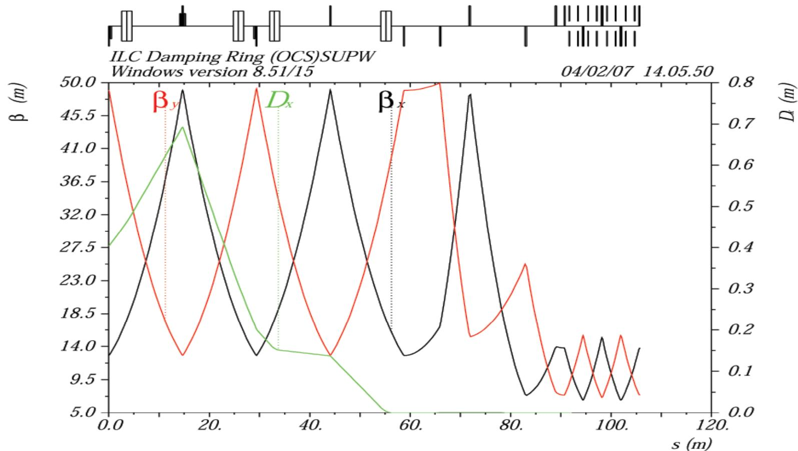
Four quadrupoles to match beta functions between arc and wiggler straight.
