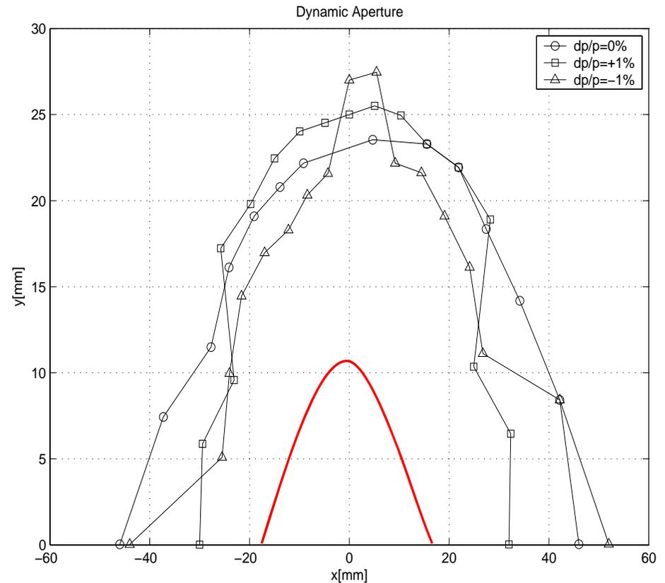
The chromaticity corrected to (0.3,0.31). The tune variation with momentum spread  $\pm 1\%$  ; the dynamic aperture with momentum spread up to  $\pm 1\%$  (with RF cavity, no errors).
