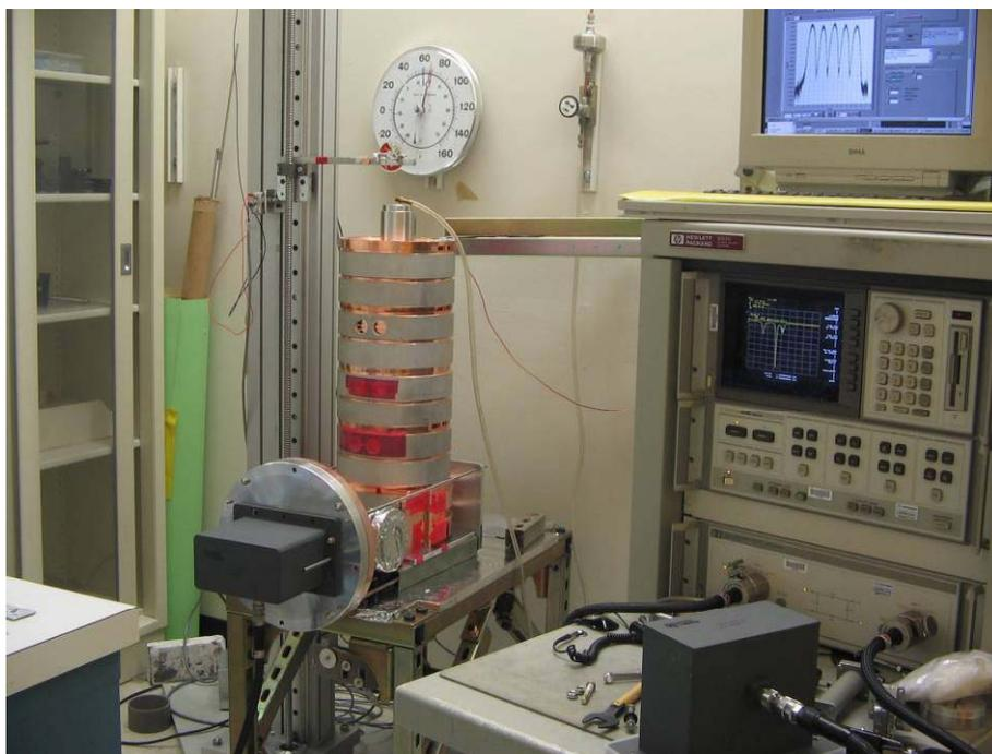
Field Plots for Bead Pulling Two Different Frequencies Showing the Correct Cell Frequency and Tuning Property.
