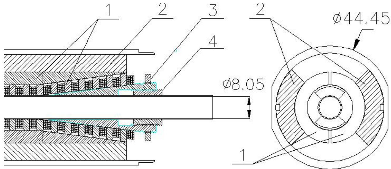
Fig.2:Details of design. 1–Iron yoke, 2–Copper collar, 3, 4–trimming Iron nuts. Inner diameter of **Copper** vacuum chamber is 8mm clear.
