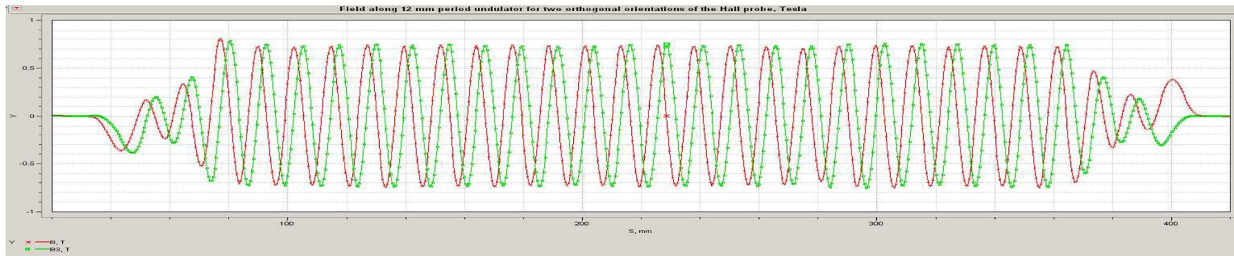
Fig.3: Field profile – conical ends. 6 layer, 12 mm period – orthogonal hall probes. 1Tesla full scale
