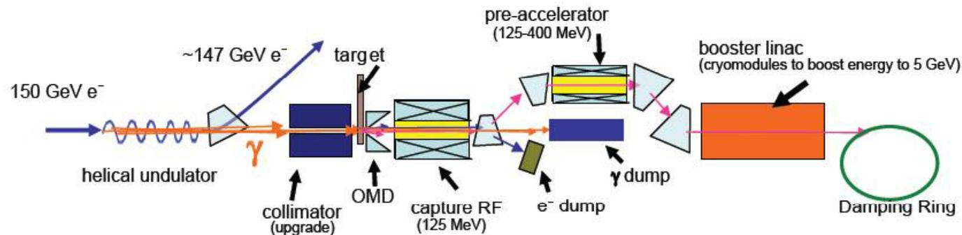
FIGURE 2.3-2. Overall Layout of the Positron Source
