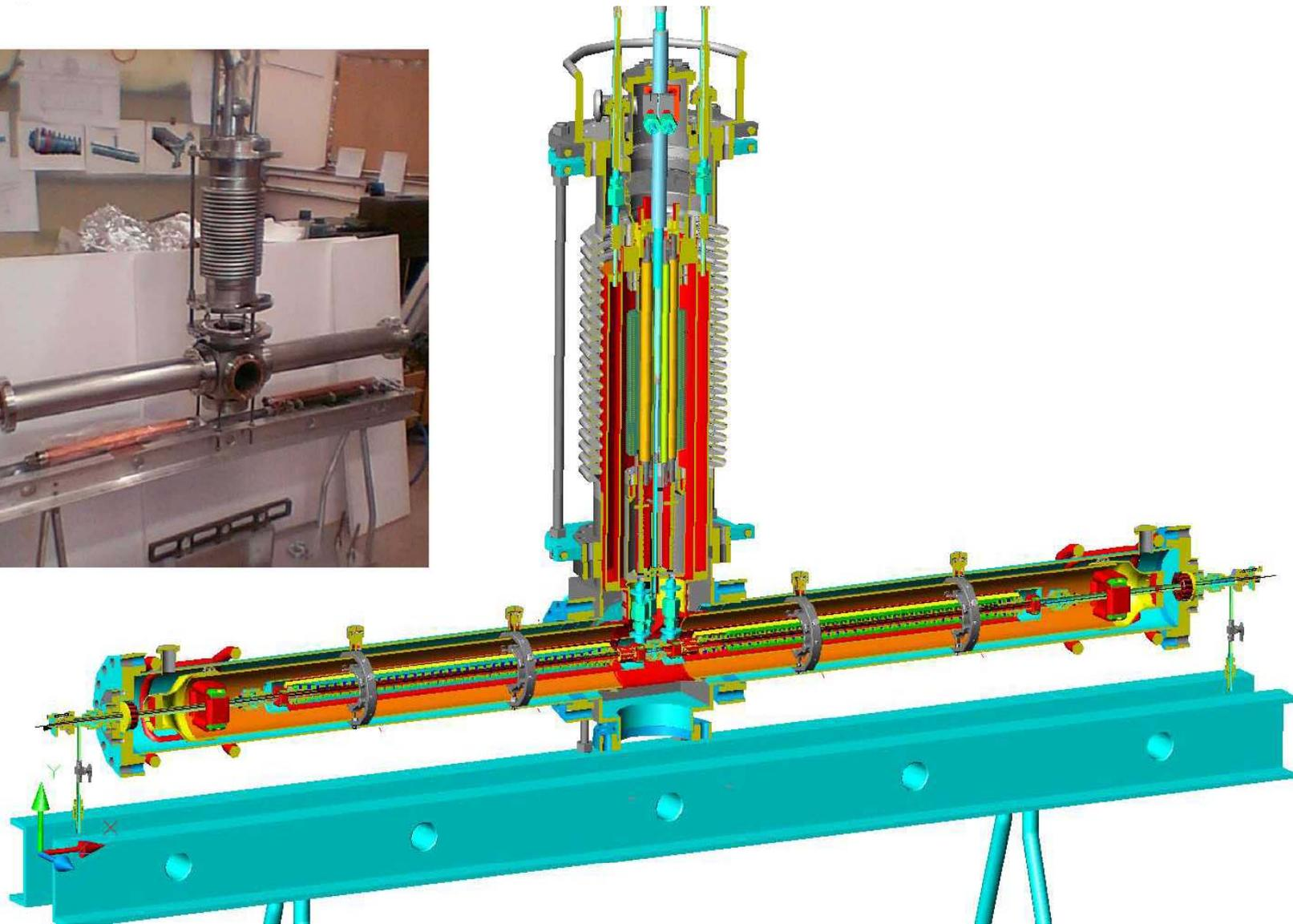
Fig.1; Extensible prototype concept for ILC positron undulator . Diameter of cryostat = 102mm
