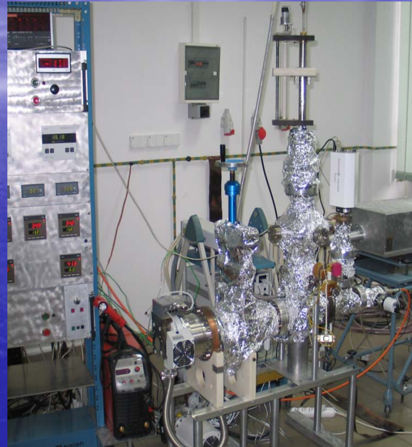
Scheme of the UHV system with a linear (cylindrical) arc and the first linear-arc facility constructed at IPJ in Swierk, Poland, in 2005.
