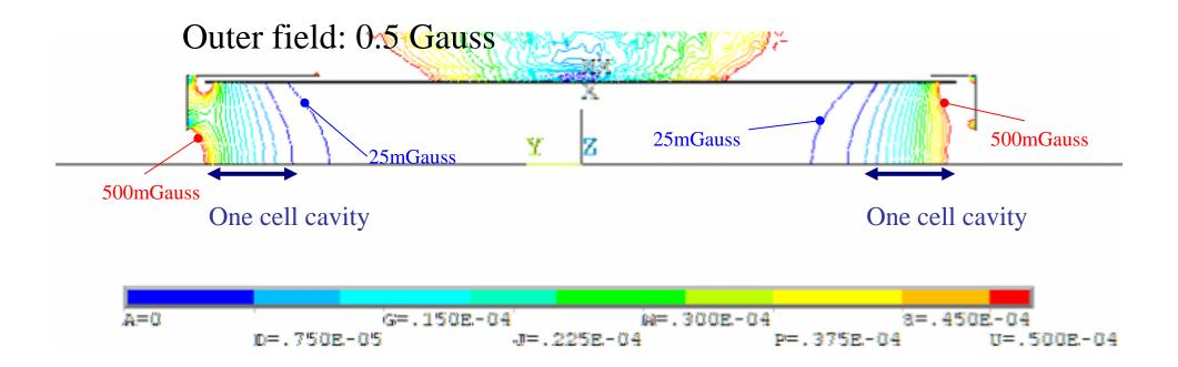
• In case of the outer field of 0.5 Gauss, the cavities in the both ends will be in the field from 0.05 Gauss to 0.5 Gauss.
