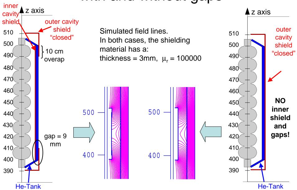
The outer shield "closed" solution: with and without gaps Comparing the two cases
