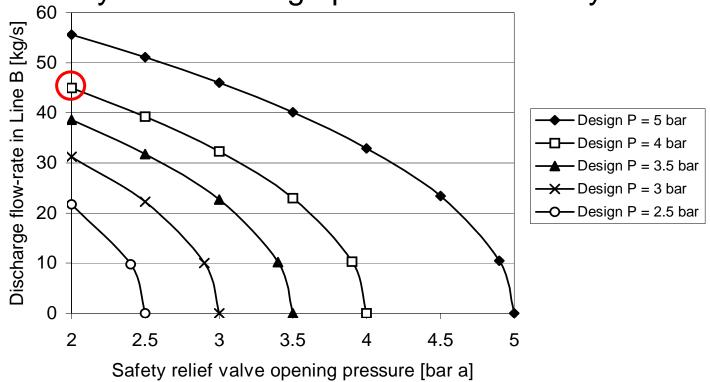
A design pressure of 4 bar at cold allows a discharge flow of 45 kg/s with a SV opening pressure of 2 bar -> i.e. a factor of about of 2 w/r to the worst case scenario
