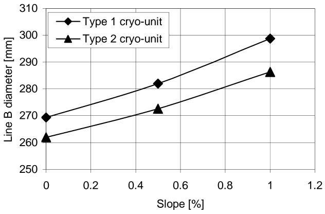
Line B designed for cavity temperature spread of 50 mK: 300 mm acceptable for slope up to 1 % Line A: 60 mm required for cavity cool-down
