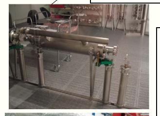
Assemble dressed Cavities to form a String in the Cavity String Assembly Area (Clean Room)
