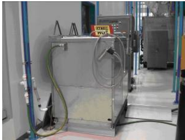
Figure 5.6: Ultrasonic cleaner to clean outer surfaces of the dressed cavities
