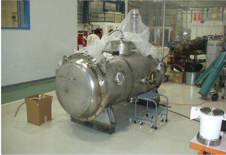
Figure 4.1 Cryostat for first HTS system under construction
