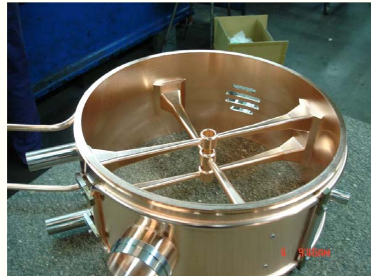
Brazed cavity before welding end walls
