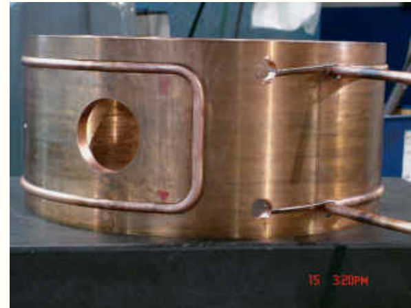
Body wall roughed in and annealed.
