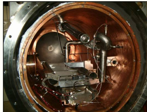
Horizontal Test Cryostat in preparation for 1 st cooldown
