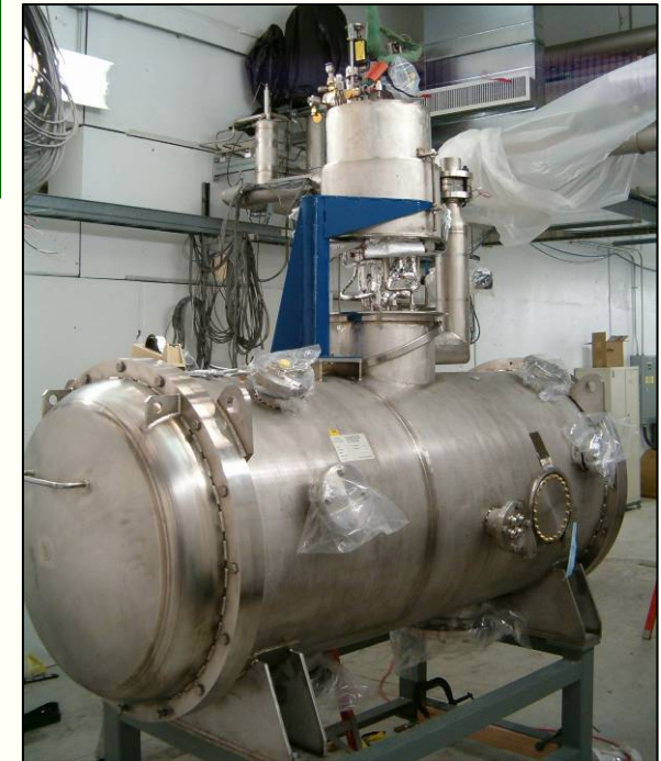
Horizontal Test Cryostat in preparation for 1 st cooldown
