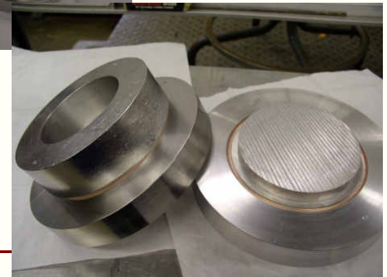
Beam pipe and power coupler brazed transitions (ANL)
