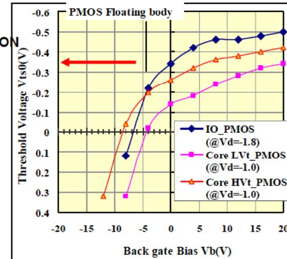
Substrate voltage acts as a back gate bias and changes the transistor threshold - like another gate
