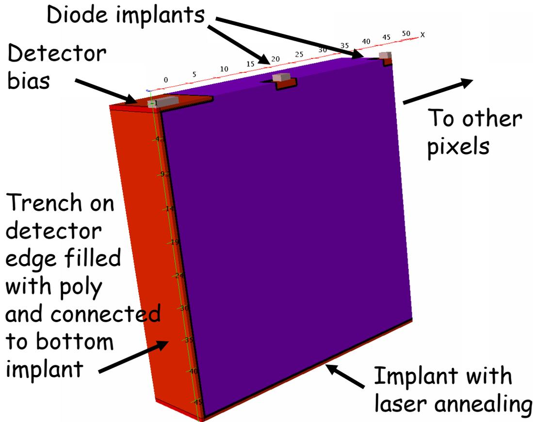
Detector Cross section near one detector edge
