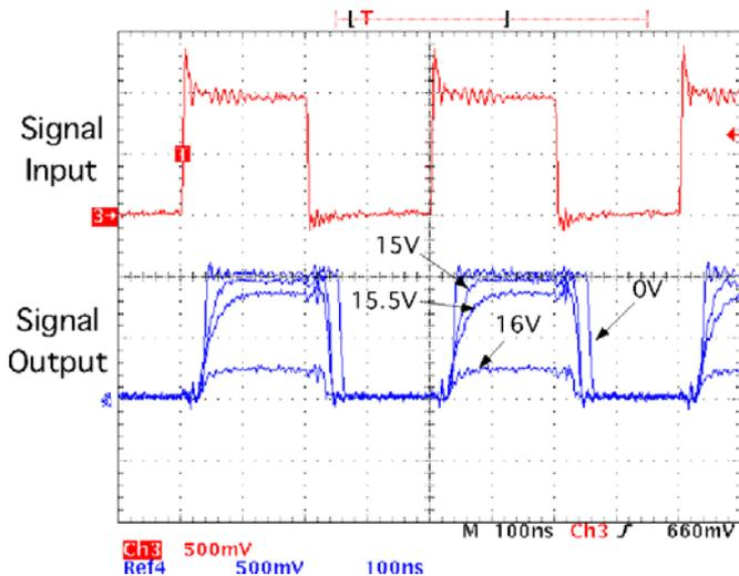
Signal disappears at  $V_b \sim 16V$
