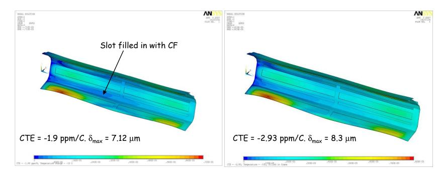
For this modified structure the maximum deflection vector goes from 8.2 to 7.12  $\mu$ m with this change in CTE. For reference the CTE for silicon is 2.49 ppm/K
