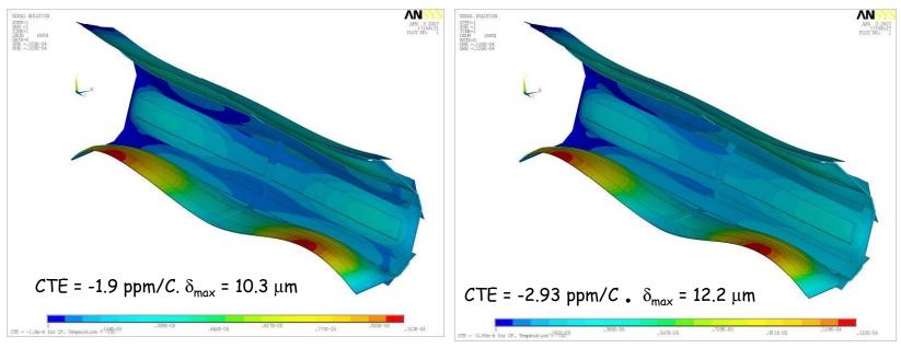
The maximum deflection vector for a 10C delta T goes from 12.2 to 10.3  $\mu$ m with this change in CTE. For reference the CTE for silicon is 2.49 ppm/K
