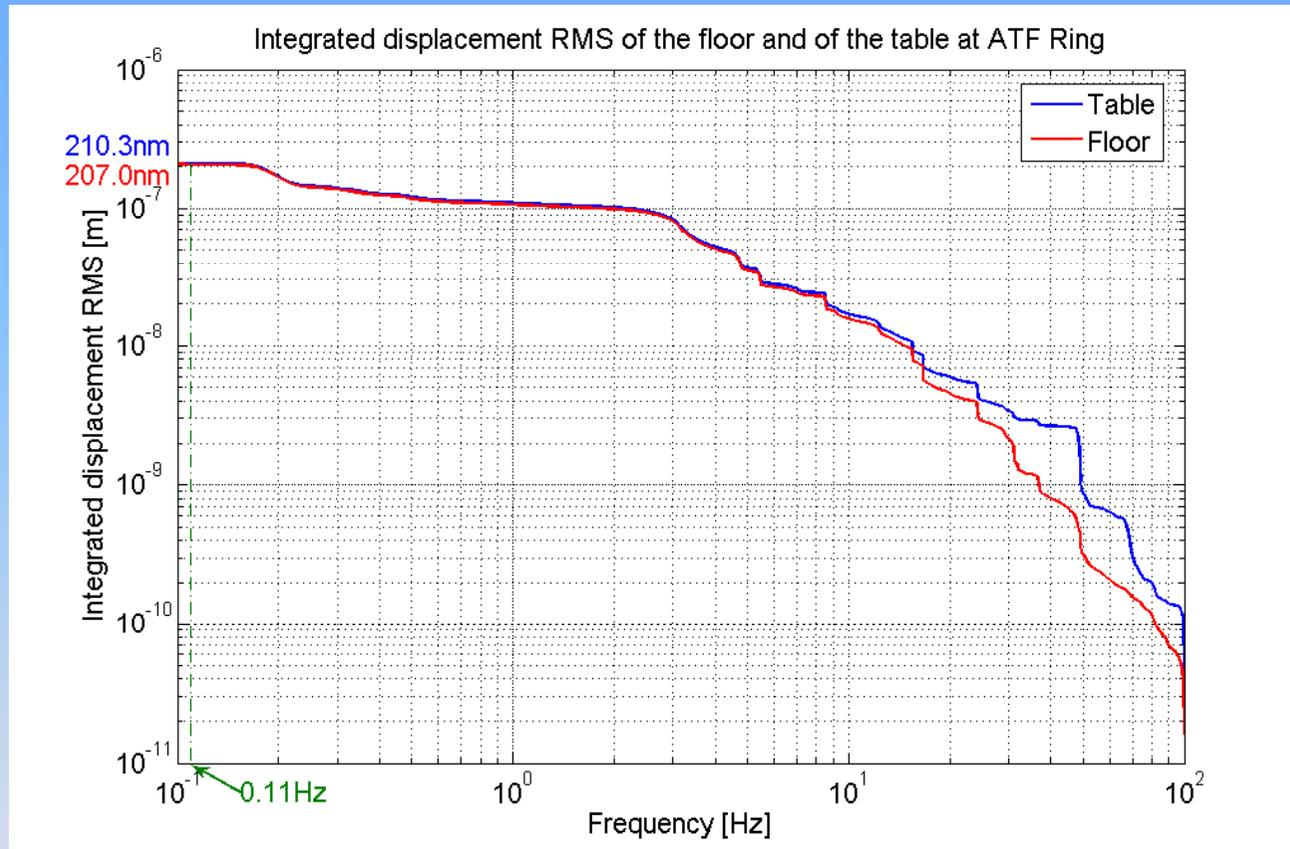
✓ Difference of integrated displacement RMS from 0.1Hz to 100Hz: 3.3nm!!!
