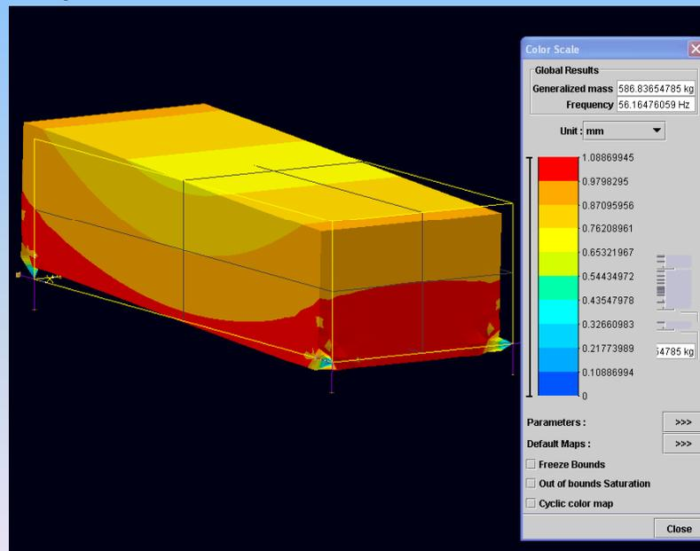
✓ Other eigenfrequencies: 58.1Hz, 58.6Hz, 76.0Hz, 85.4Hz, 95.4Hz, 248.1Hz...
