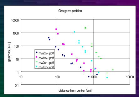
Distribution of beam halo depends on number of sigma rather than absolute distance from center (i.e.,if beam center is expanded, halo is also expanded)
