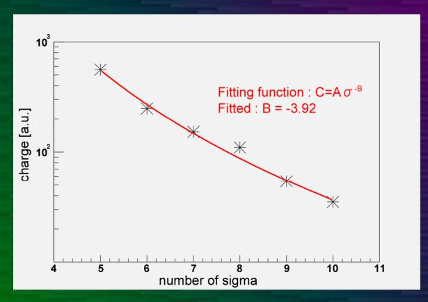
Gaussian distribution damps a factor of 1000 for every sigma, but it only damps ~σ<sup>-3~5</sup>
