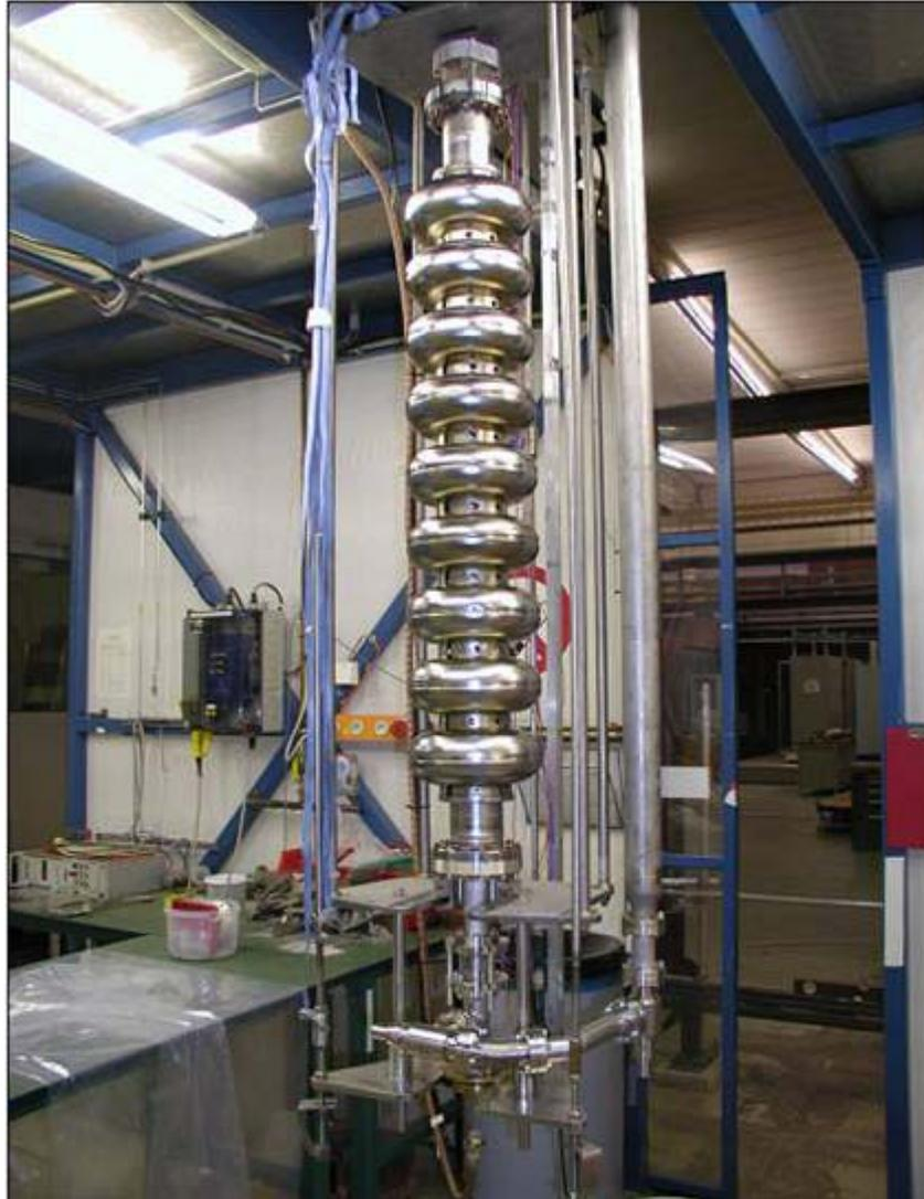
**Cavity in test insert
