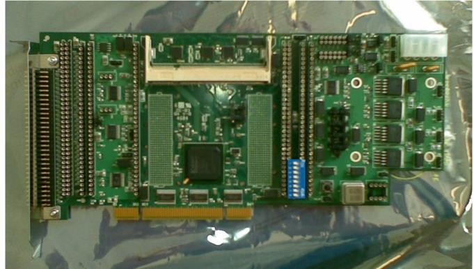
Board has DDR2 SO-DIMM socket, allowing us to install ram for event buffering. The size of the ram needed is currently not determined.
