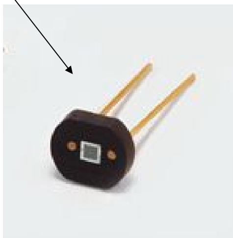
MultiPhoton PixelCounter (MPPC): Active area 1 x 1 mm, pitch 100 \mu\text{m} , ceramic package
