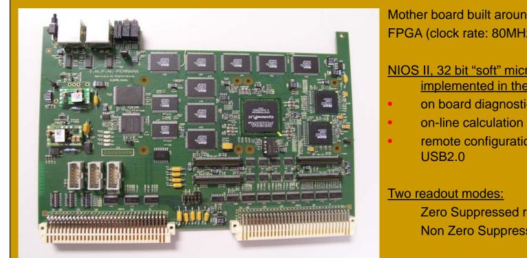
Mother board built around an ALTERA Cyclonell FPGA (clock rate: 80MHz)
