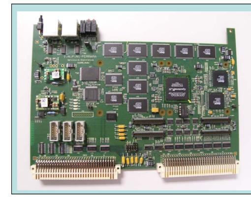
mother board built around an ALTERA Cyclonell FPGA (clock rate: 80MHz) and hosting the core resources and Interfaces (VME64X slave, USB2.0, EUDET trigger bus)
