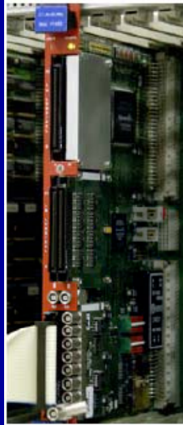
C.A.E.N. V1495 general purpose I/O module
