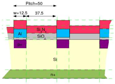
Any discontinuous and repetitive structure produces a beam diffraction:
