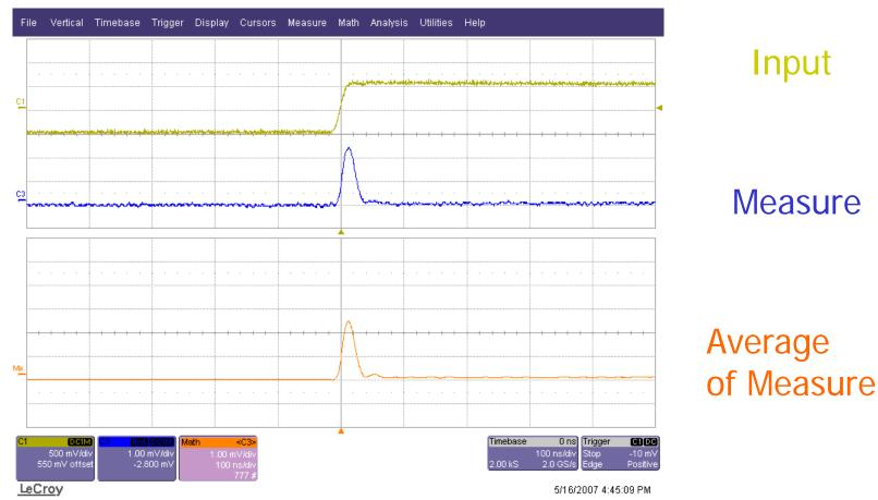
PCB 6 Layers : 2 parallels paths Hardroc Pin 2-3 (50 Ohms to GND) Pad 6-8 Input on Rpc Pad = 1VMeasure = 3.5 mV
