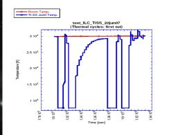
• Performed seven cycles between 300 K and 77 K with the same sample configuration (no bag)
