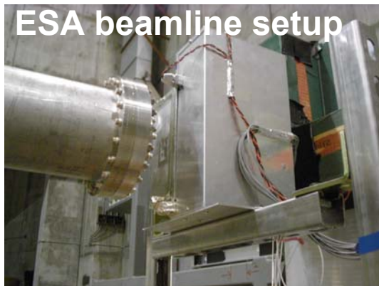
Local DAQ board w/ FPGA; fiber bundle to detector, and USB to local PC w/ ethernet
