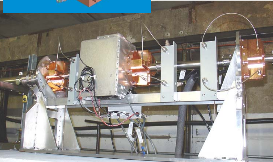
New Linac BPM Prototype (C. Adolphsen, G. Bowden, Z. Li) → used as BPM3-5 for T-474
