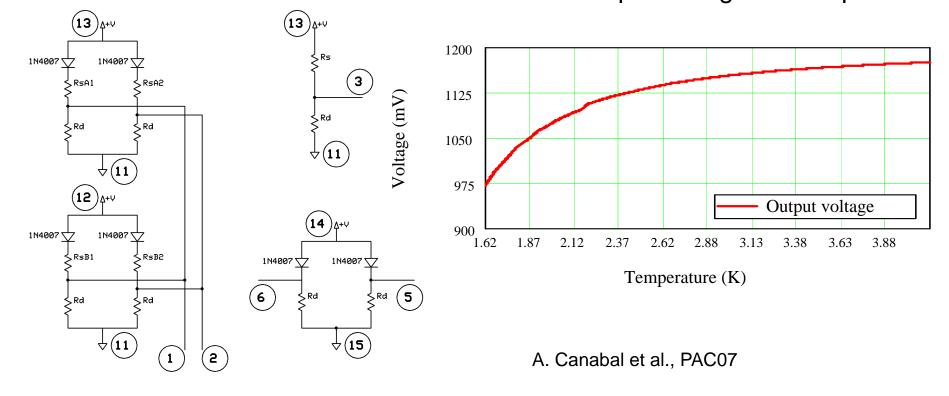
Estimated output voltage vs. temperature
