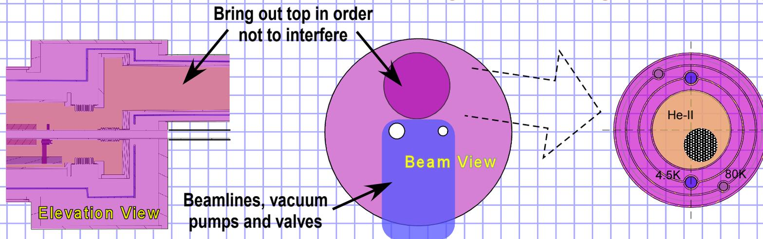
What is our budget for the space taken up by vacuum pumpout lines and the beam isolation valves? Must define relationship between cryogenic connection to QDO cryostat and other such equipment in this area.
