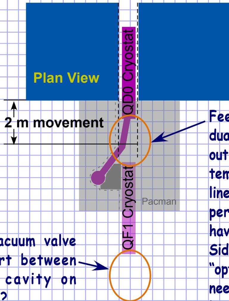
Feedback kicker, BPMs, two sets of dual beamline vacuum valves and pump out ports must fit in this space. Is a temporary roughing pump out vacuum line connection enough or do we need permanently attached lines that also have to penetrate the pacman shielding. Side comment: what about discussion of "optical anchor" where there may be a need for some optical penetrations for laser beams?
